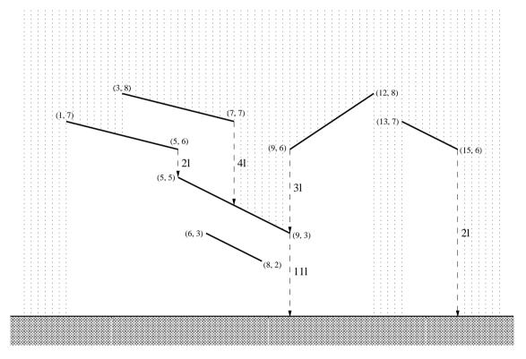
For the purpose of designing a piping system it is desired to compute how much water is flowing down from each segment of the roof. To be prepared for a heavy November rain you should count one liter of rain water falling on a meter of the horizontal plane during one second.
